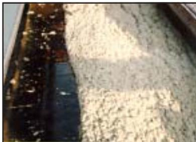
Sludge being discharged into a screw conveyor.
