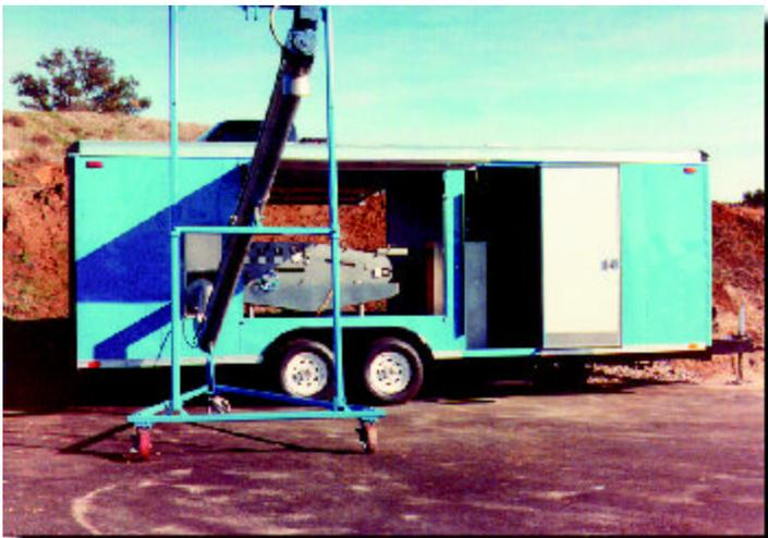
1.5 meter, stainless steel, trailer mounted belt press with auxiliary equipment
